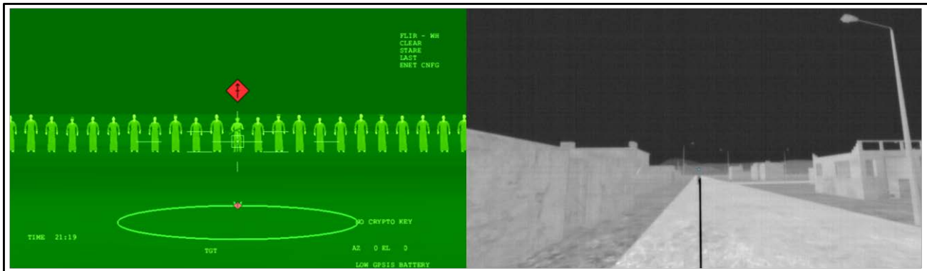
Figure 5: Human machine interface for target acquisition simulations. Our previous target acquisition task utilized a reticle at a fixed point in the center of the screen (right). We are developing ways to visualize the way a wireless controller is pointing into a virtual scene in the VPH (right). In the current VPH interface, a black beam radiates out from the users point of view towards the virtual entity being selected.
