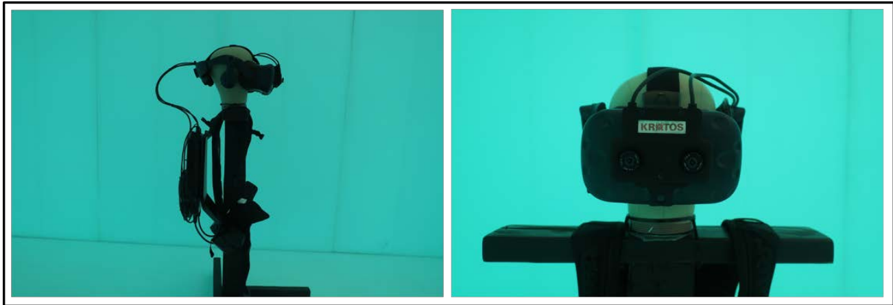
Figure 2: The wearable backpack computer system and the modified Vive display rest on a holding rack (left). A pair of cameras integrated into the Vive display enables the research team to display real objects in an otherwise virtual world (right).
